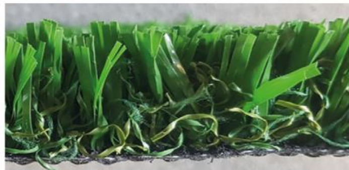
Innovative textile structure for the turf system with stabilizing yarns
