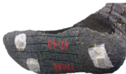
(a) Integrated textile pressure sensors with connecting measurement lines
